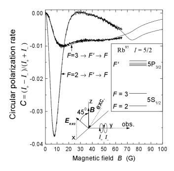
Figure 1. Calculated and experimentally recorded fluorescence circularity signals for Rb<sup>85</sup>, experimental geometry and a schematic HFS energy level diagram.
